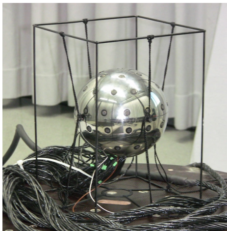
Figure 1: An experimental 64-channel microphone array with a size similar to that of a bowling ball (photograph by Karim Helwani)
